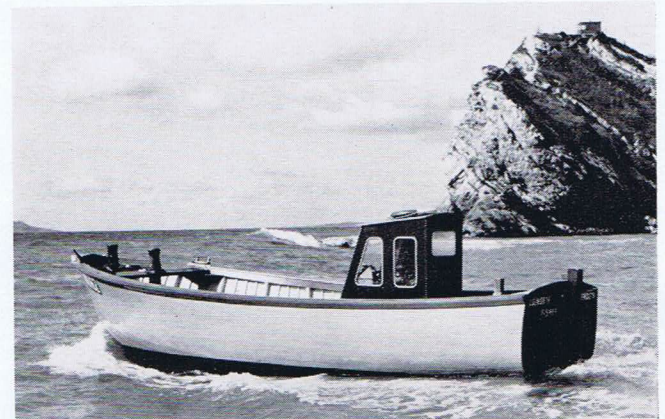
The Lulworth Fisher powered by a Petter PJ3W watercooled diesel unit. The engine is also used to drive the capstan for net hauling.
