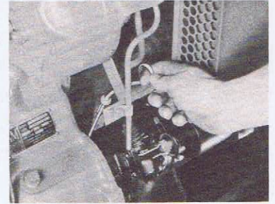
CHECK OIL LEVEL
