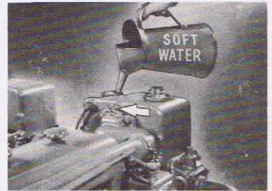
FILL COOLING SYSTEM
