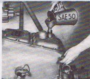
20. TWIN DISC, FILL AND CHECK
