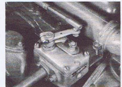
NO FUEL POSITION— LIMITING SPEED GOVERNOR
